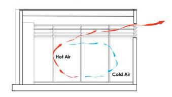
Convection removes hot air to the exterior environment in the absence of wind breezes, thus lowering the indoor dry bulb temperature. The louvered windows increase the rate of hot air replaced by cool air within CoDA
