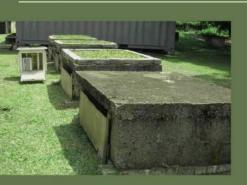
An experiment conducted by the University of Moratuwa, Sri Lanka (a tropical climate nation) indicates that houses experience a maximum outdoor and indoor temperature of 32 °C and 29.5 °C respectively. By implementing the green roof system, the outdoor and indoor temperatures are decreased by 8 °C and 3 °C respectively.
