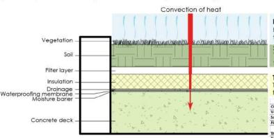
The thermal insulation layers contribute to the high thermal resistance of the green roof, thus lowering the U-value of the roof by 0.49233 W/m²k
