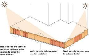
At months of the equinoxes, the North and West facades which are not shaded are fully exposed to solar radiation. The wall surfaces not only allow heat to radiate into the interior, but will also conduct heat from the hotter external environment into the cooler internal environment
